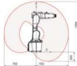
ABB IRB 1200 - SIX AXIS ARTICULATED ROBOT MANIPULATOR
