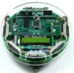
Fire Bird V ATMEGA2560 Robotic Research Platform
